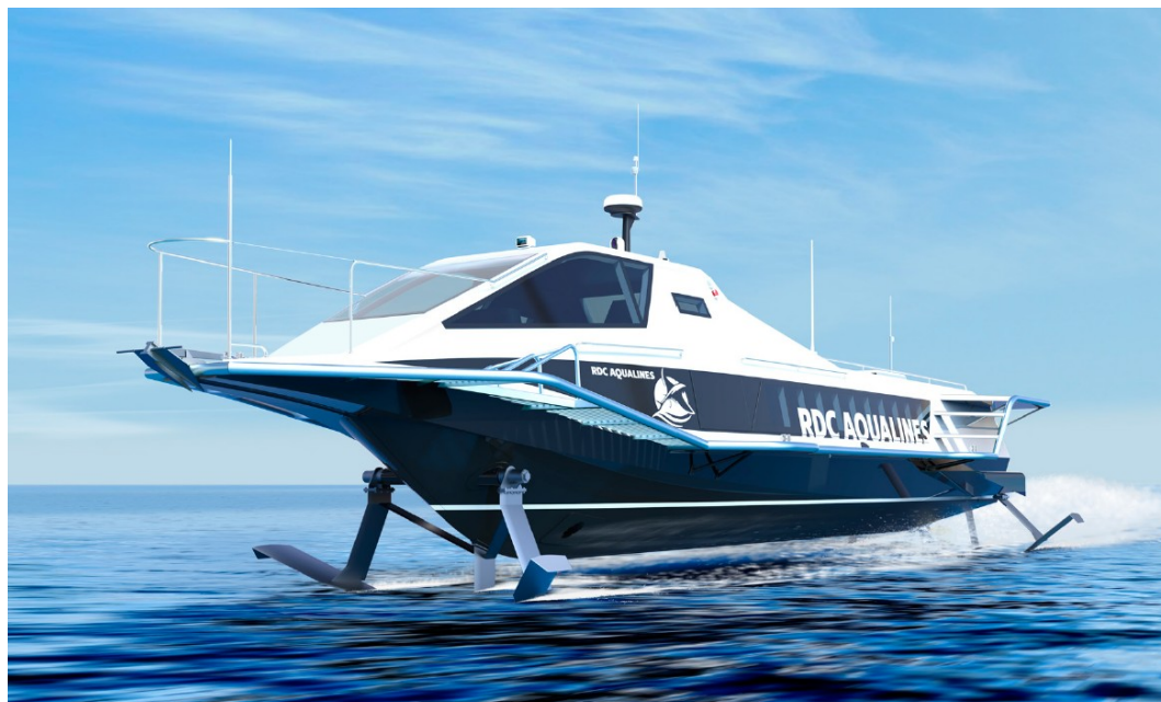
A-902 RETRACTIBLE HYDROFOIL VESSEL Hydrofoil vessel for passenger and cargo transportation in coastal regions
